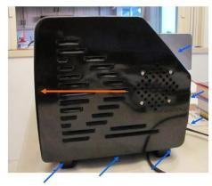
Remove 6 screws (blue arrows), slide panel forward (orange arrow) set panel aside
